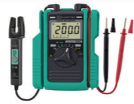
Multi Tester Digital - TA452EJ DC Volt : 340 Mv /3.4/34/340/600 V AC Volt : 3.4/34/340/600 V Resistensi : 340Ω/3.4k/34k/340k/3.4M/34M Ω Konduksi : Buzzer sounds when 30 ± 10 Ω or less Frekuensi : (Current) 3.4 k / 10 kHz (voltage) 3.4 k / 34 k / 300 kHz Batteries : AAA batteries R 03 (1.5 V) x 2 - W 87 x D 21 x H 128 mm - about 210 g
