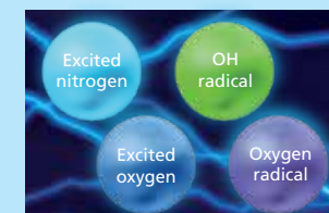
The electrons collide and combine with nitrogen and oxygen in the air to form four kinds of decomposing elements with decomposition power.
