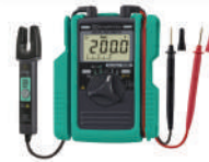
Multi Tester Digital - TA452EJ DC Volt : 340 Mv / 3.4/34/340/600 V AC Volt : 3.4/34/340/600 V Resistensi : 340Ω/3.4K/34K/3.4M/34M Ω Konduksi : Buzzer sounds when 30 ± 10 Ω or less Frekuensi : (Current) 3.4 k / 10 KHz (voltage) 3.4 k / 34 k / 300 kHz Batteries : AAA batteries R 03 (1.5 V) × 2 - W 87 × D 21 × H 128 mm - about 210 g
