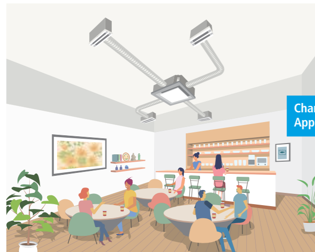
Cafe: Three airflow outlets are located in the customer area with one above the counter.
